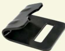
4" Flat Hook B/S: 15000lbs/6800kgs Art No. FT-100-D1 N.W.: 0.47kg
