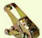
1' Standard Handle Ratchet Buckle B.S.: 3300lbs/1500kgs ArtNo. RB-025-03 N.W.: 0.35kg
