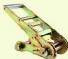
3" Long Handle Ratchet Buckle B.S.: 22000lbs/10000kgs ArtNo. R8-075-01 N.W.: 3.00kg
