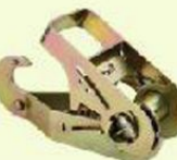
1-3/4' Ratchet Buckle w/Hook B.S.: 6000lbs/2725kgs ArtNo. RB-045-01 N.W.: 0.73kg
