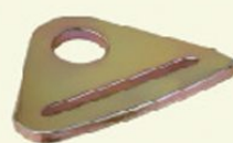
2" Connect plate S.S.: 5000lbs/2270kgs ArtNo. CP-050-01 N.W.: 0.07kg
